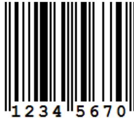
**Description:** EAN 8 is the short form of EAN-13. This code is only used if the article is too small for an EAN-13 code. The restrictions for this are very hard. An EAN-8 will only be granted if a EAN-13 will uses more than 25% of the front space of the article. An EAN-8 always has 8 digits:
