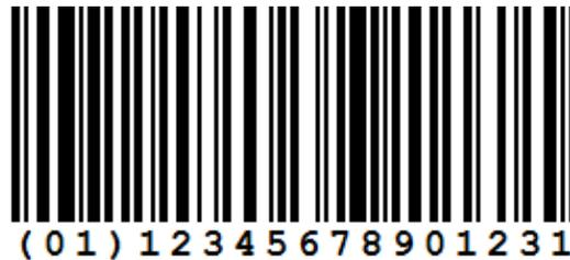
**Description:** The *DUN-14* (Distribution Unit Number) is not really a barcode type. It's a numbering system for shipping containers that uses other barcode symbology. The DUN-14 uses the ITF-14 or the EAN-14 symbol set. Modern installations always use the EAN-14 to encode the DUN-14.
