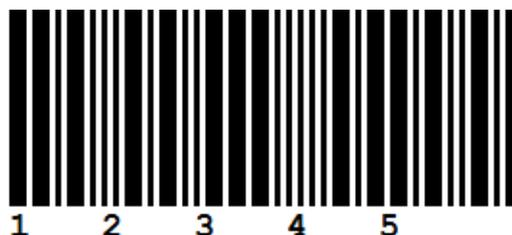
And here the same digits 123456 coded as Code 25 Interleaved:
