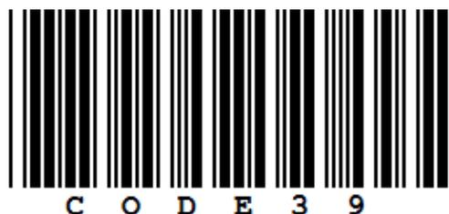
And here is the code if you use the Type "Code 39 Checksum" (#26) with a check digit calculated according to Modulo 43:
