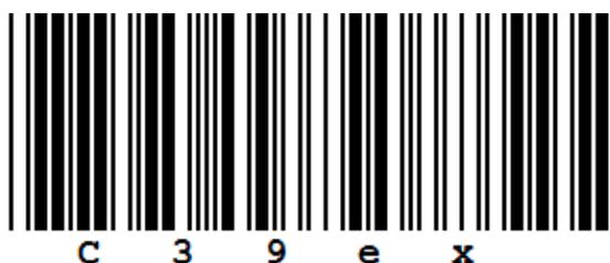
And here is the code if you use the Type "Code 39 ExtendedChecksum" (#27) with a check digit calculated according to Modulo 43:
