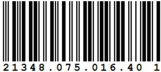
**Description:** The Leitcode is a numeric code using the numbers 0..9. This code is used by the Deutsche Post AG (DHL). The base of this code is Code 25 Interleaved, but with a different check digit.
