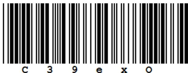
Code 39 Extended can be produced in different **proportions**: 2,0:1 and 3,0:1. This is the proportion between the thin and the thick lines of the code. As higher the proportion, the wider is the printed barcode with same contents, but even better is readability. ActiveBarcode always used the proportion 3,0:1.
