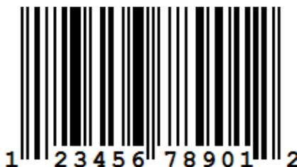
**Description:** The **UPC A** code is the standard version of the UPC code and has 12 digits. It is also called UPC 12 and is very similar to the EAN code.
