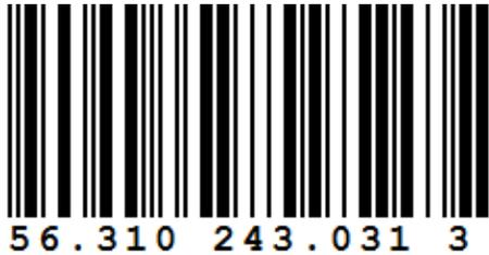
**Description:** The Identcode is a numeric code using the numbers 0..9. This code is used by the Deutsche Post AG (DHL). The base of this code is Code 25 Interleaved, but with a different check digit.
