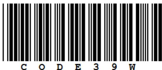
Code 39 can be produced in different **proportions**: 2,0:1 and 3,0:1. This is the proportion between the thin and the thick lines of the code. As higher the proportion,
