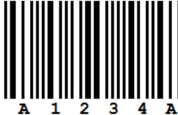
**Description:** **Codabar** is a numeric code with some additional special characters (0..9 and - \$ : / . +). There are four different start and stop signs defined. These start and stop signs are used in our software as A, B , C and D. They are only valid at the beginning and the end of the code. They can be used to transport additional information.
