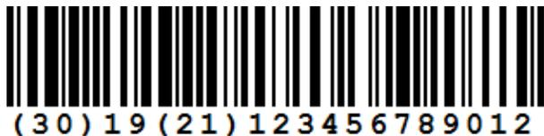
In this example the "number of parts" is 19 and the serial number is 123456789012. The "number of parts" can be up to 8 digits long. So we code a FNC1 after the 9 to let the scanner know, that the AI is closed here now and a new one follows. To create a FNC1 with ActiveBarcode simply enter <FNC1> into the text property as shown in this example:
