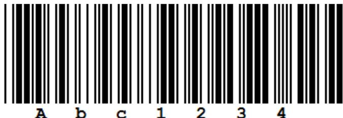
**Description:** Code 39 Extended is an extended version of Code 39 that supports the ASCII character set. So with Code 39 Extended you can also code the **26 lower letters (a-z)** and the special characters you have on your keyboard.
