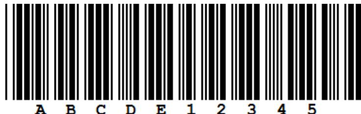
**Description:** **Code 39** is an **alphanumeric** code. Each character is built by 9 elements (5 lines and 4 spaces) where 3 are thick and 6 are thin. This allows the self checking of code 39. Code 39 does not require a build-in check digit. The main advantage is the wider character set.
